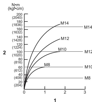
1. Fastening time (second) 2. Fastening torque
