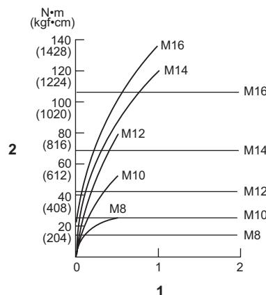
1. Fastening time (second) 2. Fastening torque
